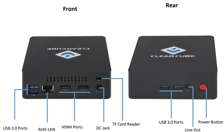
Figure 1. The CD8804 Features and Components
