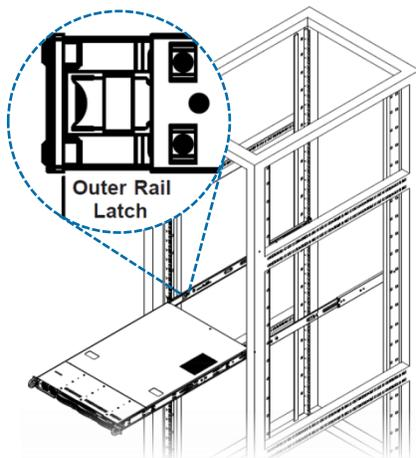
1. Press the outer rack rail latch to release the workstation chassis (the latch is shown in the adjacent picture).
